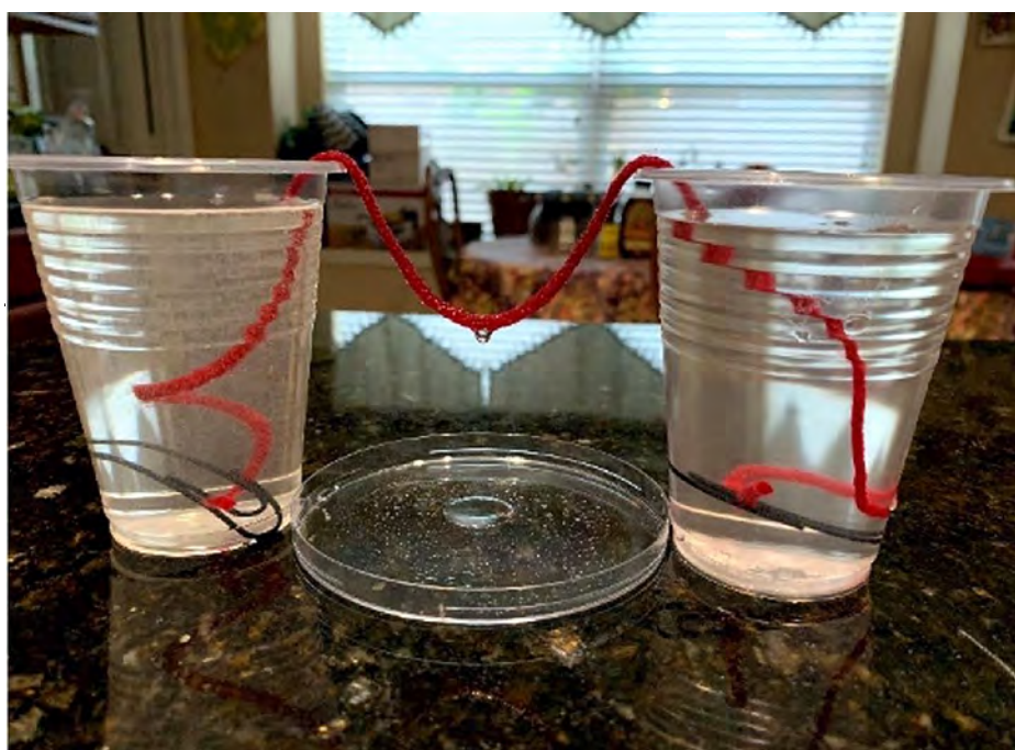
At-home experiment displays the early stage of decomposing baking soda to grow stalactite and stalagmite. The liquid (sodium carbonate solution) was made by decomposing sodium bicarbonate (baking soda) at home. PHOTO CREDIT: RIYASA SHRESTHA
